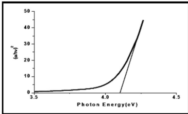
Fig. 3 band gap determination of ZnS (A).
