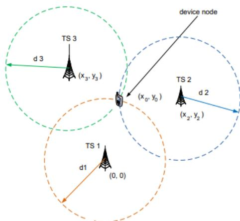
Figure 1. Illustration of the TOA method
