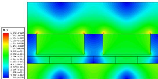
Figure 8. Flux density distribution for no-load condition of TORUS-NS machine.
