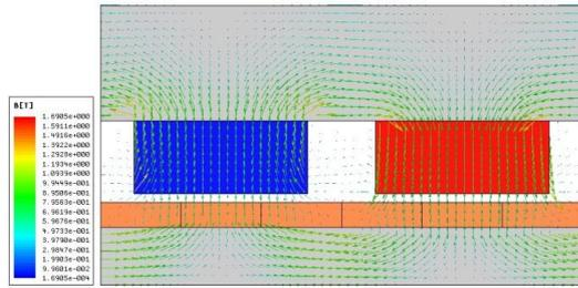
Figure 7. Flux density distribution by means of vectors and direction of flux for no-load condition.
