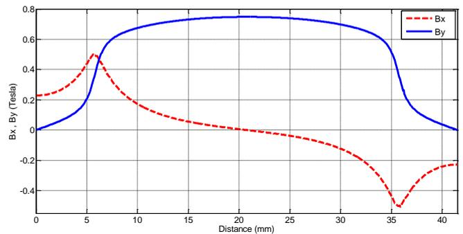
Figure 10. Magnetic flux density in the x (tangential) and y (normal) directions of TORUS-NS machine.
