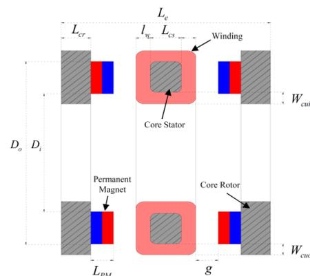
Figure 2. Definition of the geometrical parameters for the TORUS-NS AFPM machines [8]
