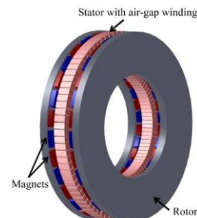
Figure 1. Axial flux TORUS type non-slotted surface mounted PM machine configuration (TORUS-NS).
