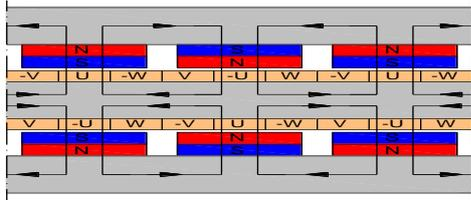
Figure 3. Three-phase winding, PM polarities and magnetic flux paths of a TORUS-NS machine [1].
