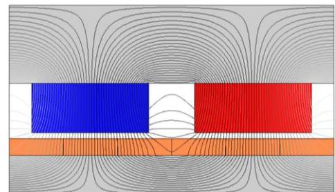
Figure 6. Magnetic flux lines for no-load condition of TORUS-NS machine.
