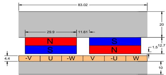
Figure 4. View of model for simulation of TORUS-NS machine.
