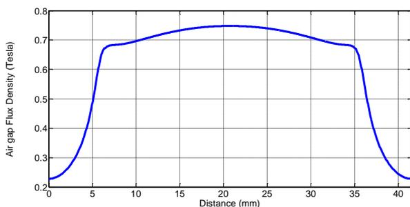
Figure 9. No load air-gap flux density of the TORUS-NS (at average diameter  $D_g = (D_i + D_o)/2$ ).
