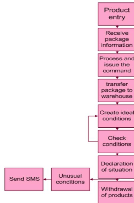
Figure5. The flowchart of proposed system
