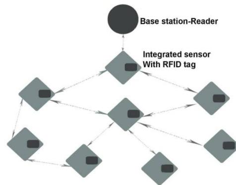
Figure2. Integrated sensor-tags that form a cooperative ad hoc network
