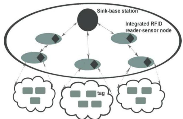
Figure3. Integrating RFID Readers with Wireless Sensor Nodes
