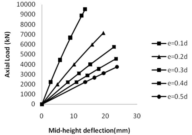
Figure 4: Load Deflection curve of  $P_b$  column with L/d ratio 15
