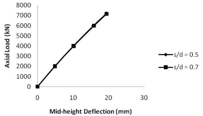
Figure 13: Load Deflection curve of  $P_d$  column with  $e/d$  0.3 and  $L/d$  15
