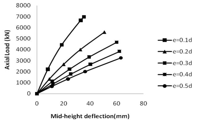
Figure 5: Load Deflection curve of  $P_b$  column with L/d ratio 25
