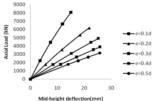
Figure 6: Load Deflection curve of  $P_d$  column with L/d ratio 15
