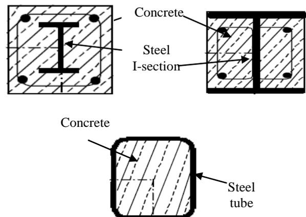
Figure 1: Typical cross-sections of (a) Fully encased composite column (FEC), (b) Partially encased composite column (PEC) and (c) Concrete filled tubular sections (CFT).
