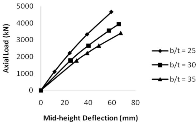
Figure 12: Load Deflection curve of  $P_b$  column with  $e/d$  0.3 and  $L/d$  25
