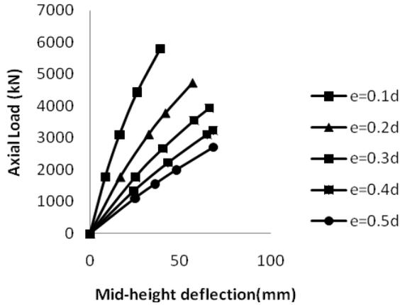
Figure 7: Load Deflection curve of  $P_d$  column with  $L/d$  ratio 25
