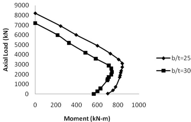
Figure 15: Variation of P-M curve with flange plate slenderness ratio
