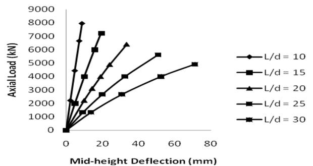
Figure 8: Load Deflection curve of  $P_a$  column with  $e/d$  ratio 0.2
