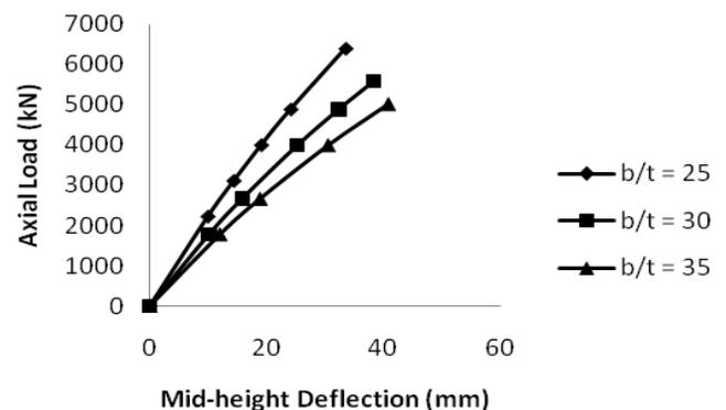
Figure 11: Load Deflection curve of  $P_a$  column with  $e/d$  0.2 and  $L/d$  20
