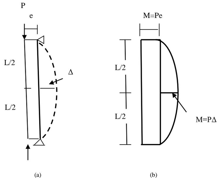
Figure 3: (a) Column subjected to eccentric loading (b) Bending moment diagram of the column
