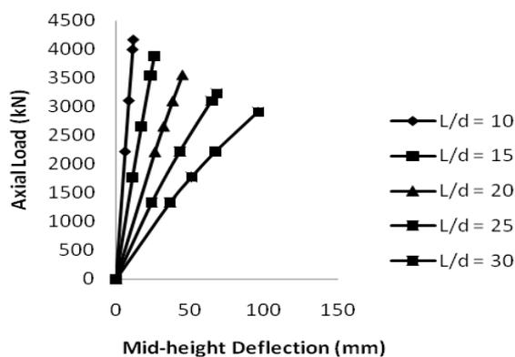
Figure 10: Load Deflection curve of  $P_d$  column with  $e/d$  ratio 0.4
