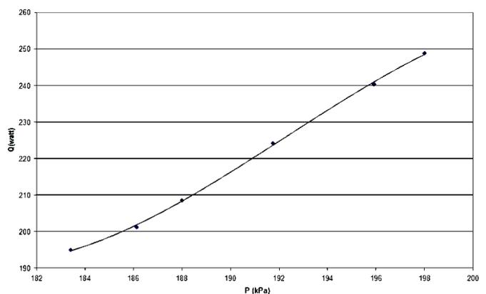
Figure 6. Variations of axial heat flux changes with saturation pressure for steady state in temperature interval 117.5-121°C
