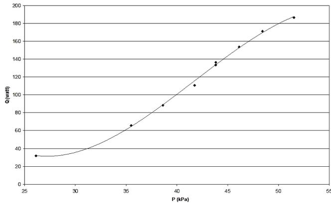
Figure 3. Variations of axial heat flux changes with saturation pressure for steady state in temperature interval 64-87°C.
