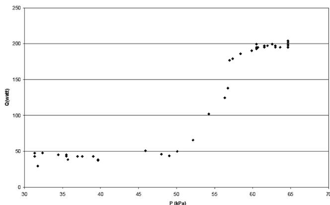
Figure 4. Variations of axial heat flux changes with saturation pressure for unsteady state in temperature interval 87.5-92.5°C
