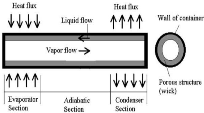
Figure 1. Conceptual drawing and operation of a conventional heat pipe [8].
