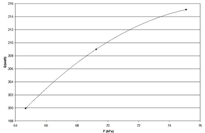
Figure 5. Variations of axial heat flux changes with saturation pressure for steady state in temperature interval 87.5-92.5°C
