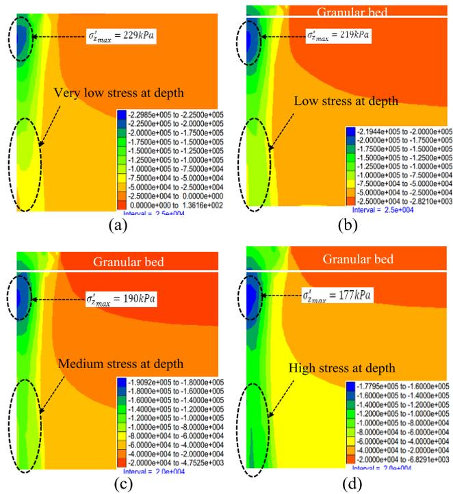
Figure 8. Effective stress contours for different thickness of granular bed at pressure of 100 kPa: a)  $t = 0$ , b)  $t = 0.15 D_f$ , c)  $t = 0.25 D_f$ , d)  $t = 0.35 D_f$
