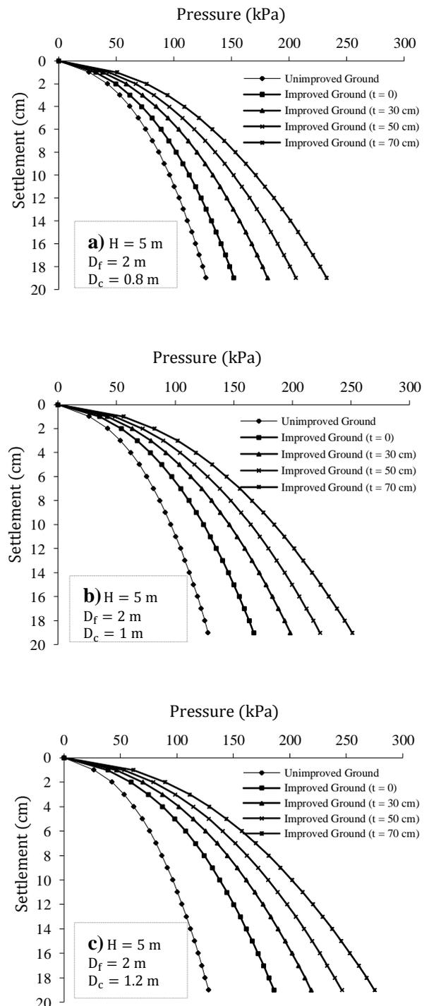
Figure 4. Pressure versus settlement curves for different diameters of stone columns: a)  $D_c = 0.8$  m, b)  $D_c = 1$  m, c)  $D_c = 1.2$  m
