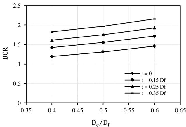
Figure 5. BCR versus the  $D_c/D_f$  for different thickness of granular bed at settlement of  $0.1 D_f$
