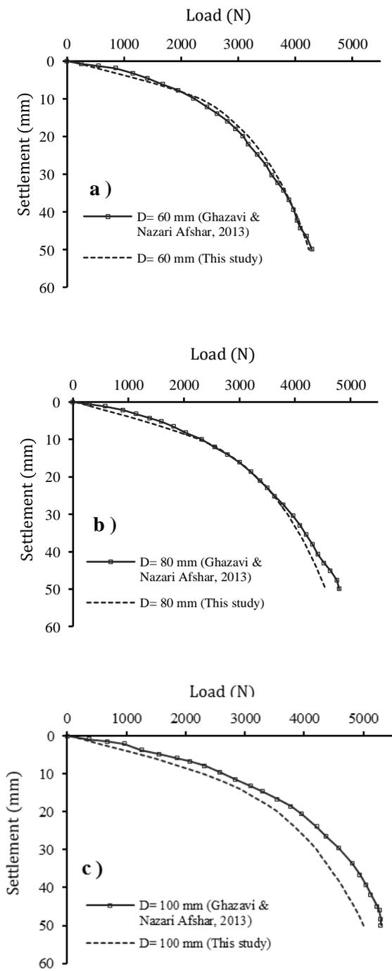
Figure 3. Validation of numerical model by results of [18]: a)  $D_c = 60$  mm, b)  $D_c = 80$  mm, c)  $D_c = 100$  mm
