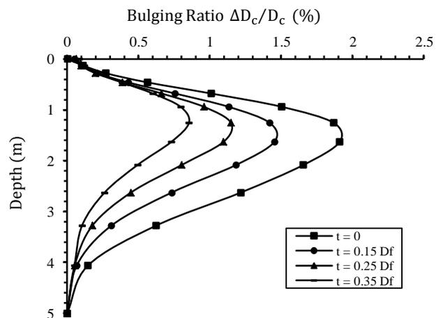
Figure 7. Bulging ratio versus the Depth for different thickness of granular bed at pressure of 100 kPa
