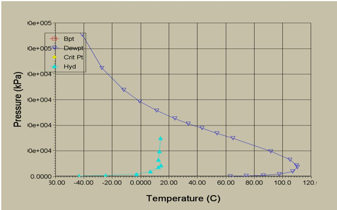
Figure B5: Hydrate Curve for Reg. feed
