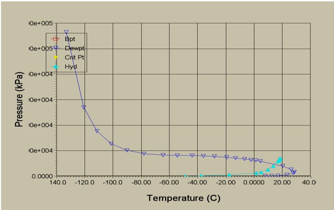
Figure B2: Hydrate Curve for GDC feed
