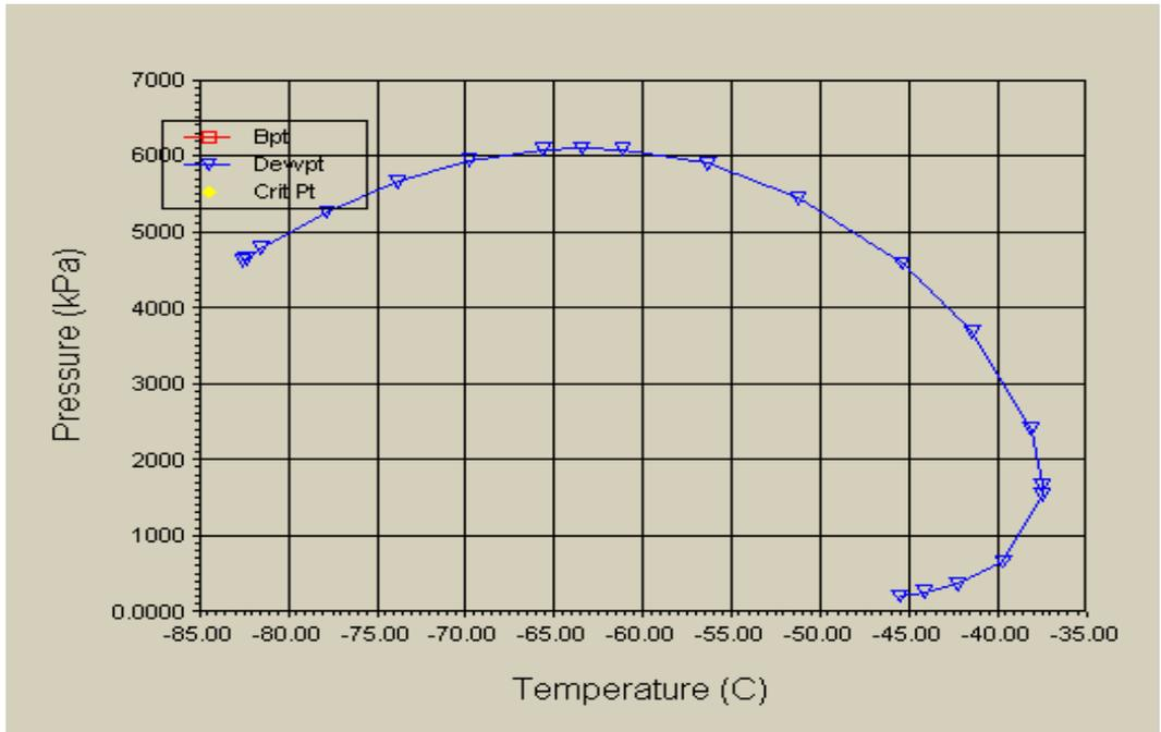
Figure B3: Hydrate Curve for GTL feedgas
