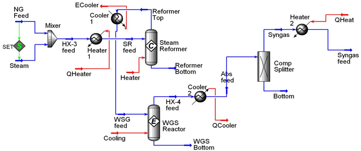
Figure 2. Process Flow Diagram of Stage 2.
