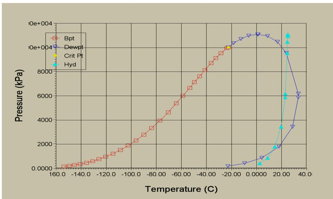
Figure B1: Hydrate Curve for GS feed
