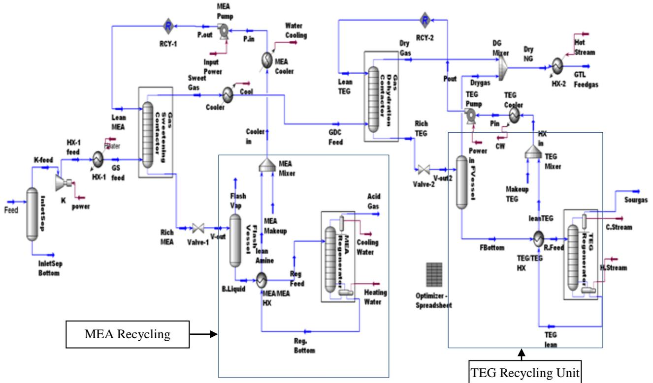
Figure 1. Process Flow Diagram of Stage 1
