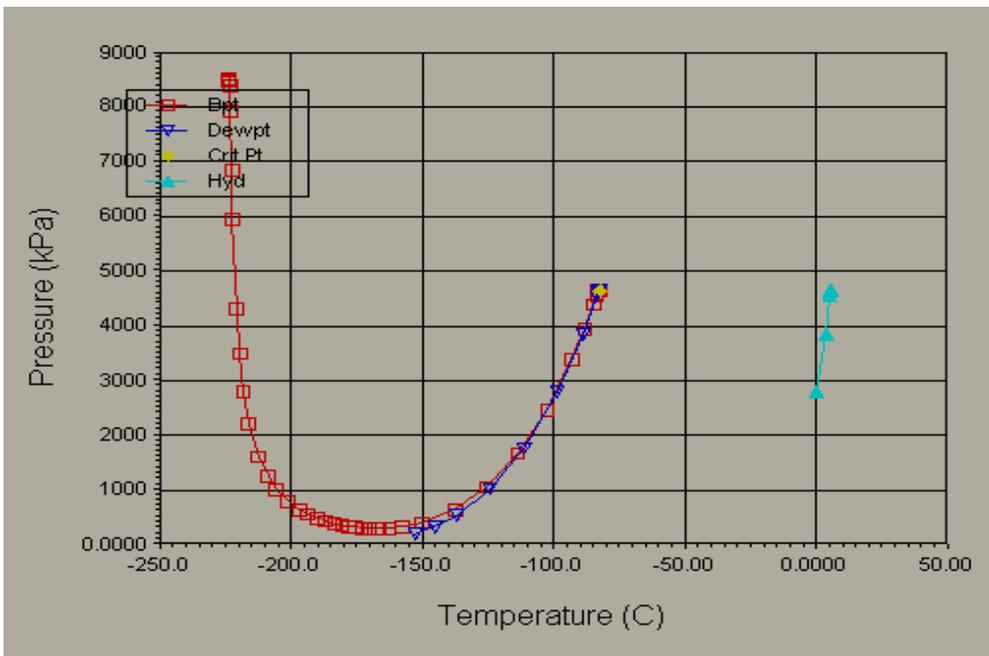
Figure B7: Hydrate Curve for WGS feed
