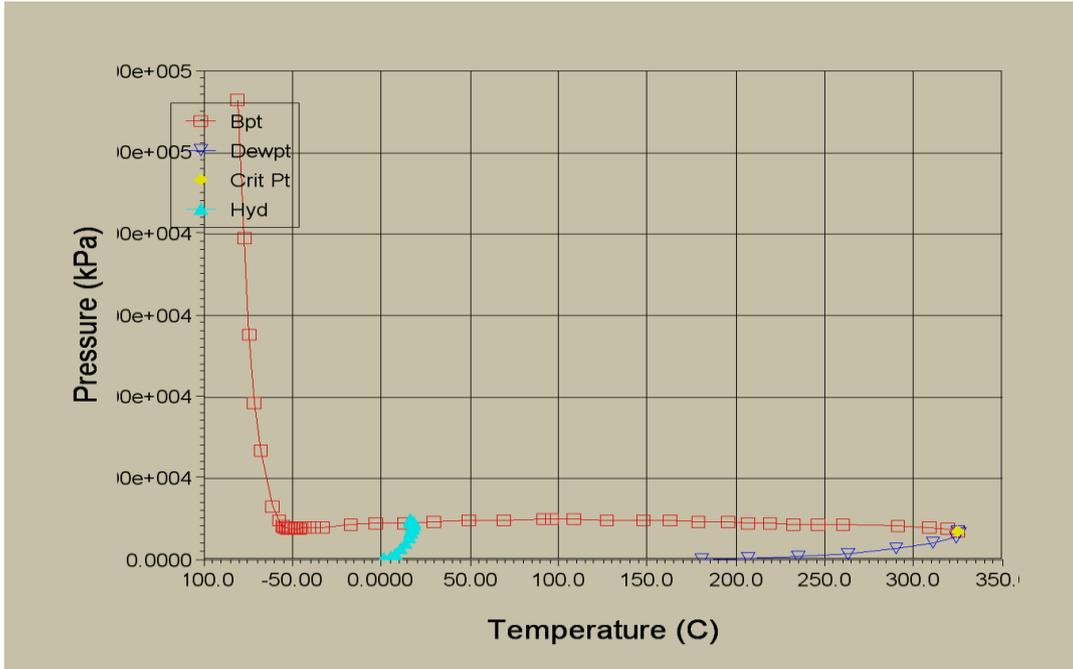
Figure B4: Hydrate Curve for R. feed
