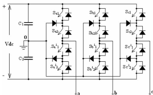
Figure 4. 3-level NPC inverter
