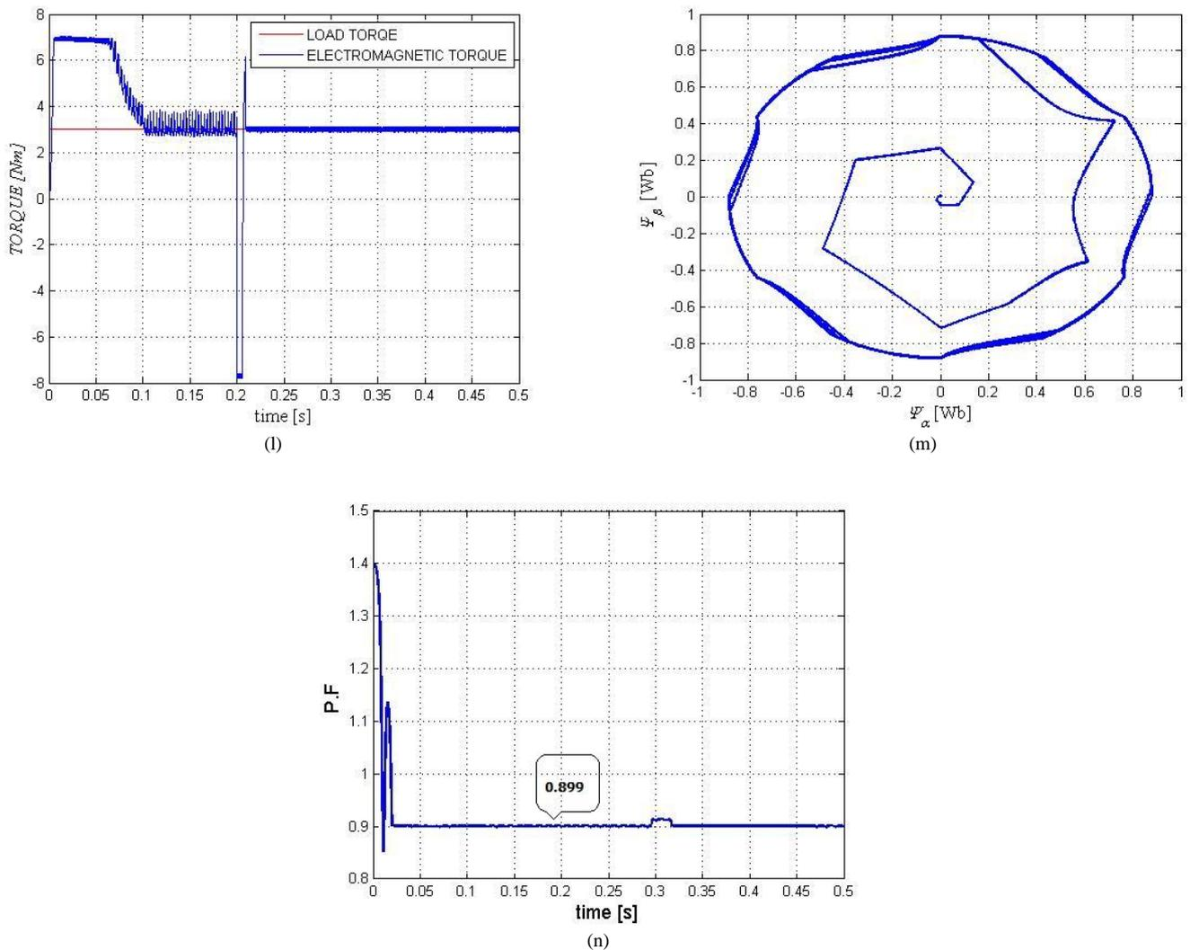
Figure 10. DTC-SVM without PFC (h) input voltage, (l) input current, (j) dynamics stator current, (k) speed response, (l) performance of torque, (m) locus of stator flux, (n) power factor without dual boost converter.
