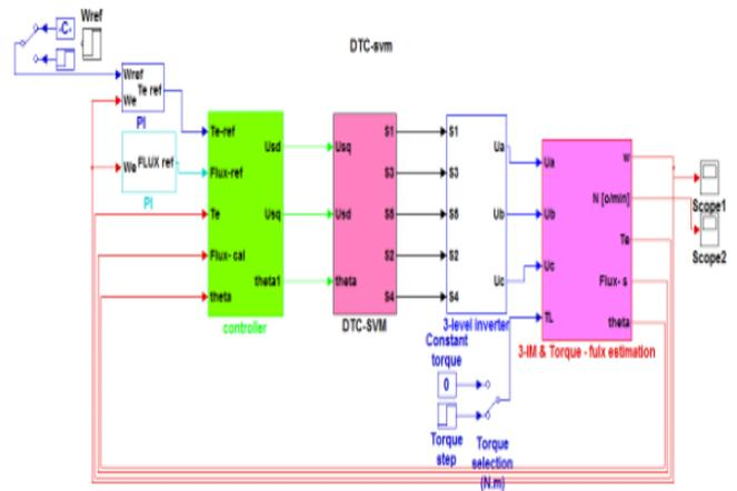
Figure 8. Overall Proposed DTC-SVM Of Motor.
