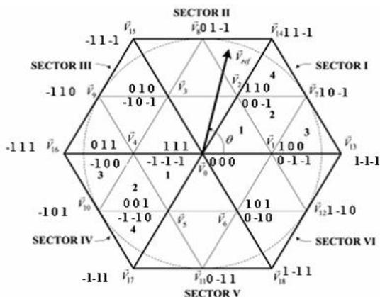
Figure 5. Vector map for three levels NPC.
