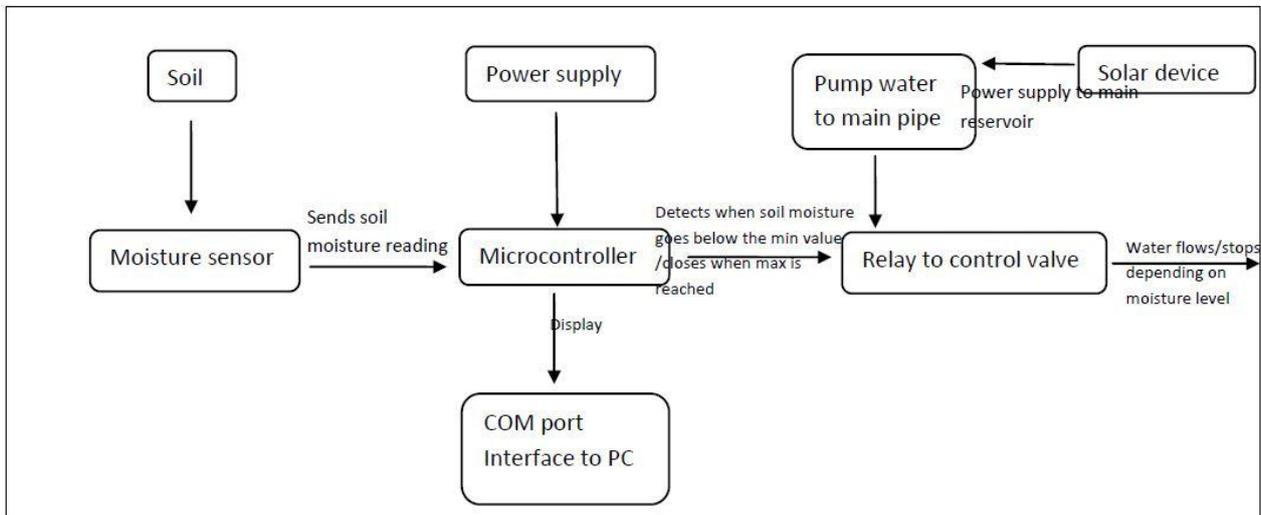
Figure 1. Components of auto watering irrigation system [7]
