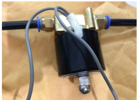
Figure 7. Automated on/off valve
