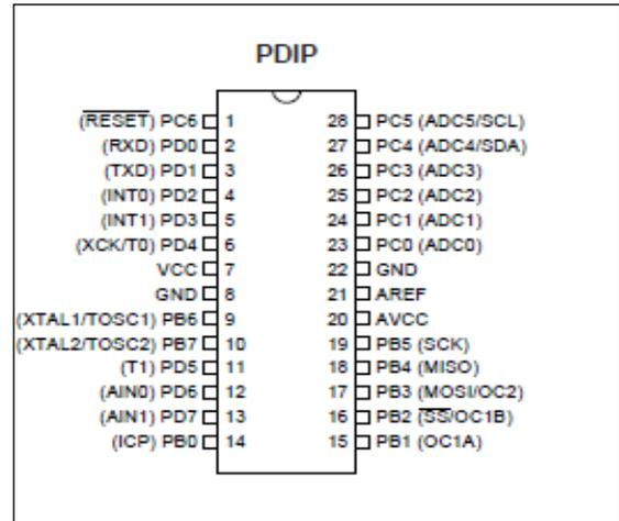
Figure 9. MEGA 8 AVR pin diagram
