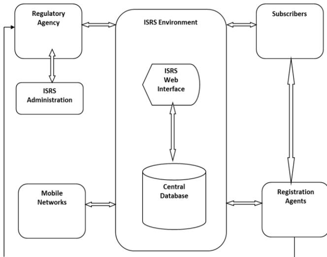
Figure 1. High Level Model of the Integrated SIM Registration System
