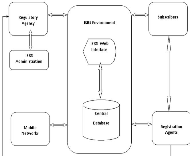
Figure 3. Architectural Design of the Integrated SIM Registration System
