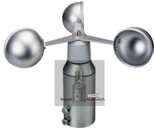
Figure 11. Three – cup anemometer
