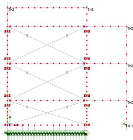
Figure 16. Numerical simulation of the three story masonry infilled R/C frame with equivalent diagonal struts
