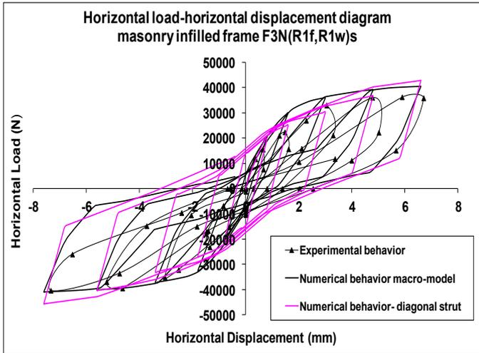
Figure 5. Comparison of cyclic response for specimen F3N(R1f,R1w)s
