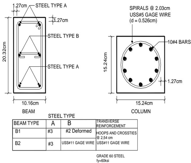
Figure 12. Column and beam design details (American reinforcement details)
