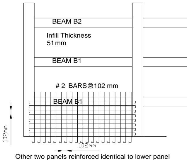
Figure 13. Masonry infill reinforcement
