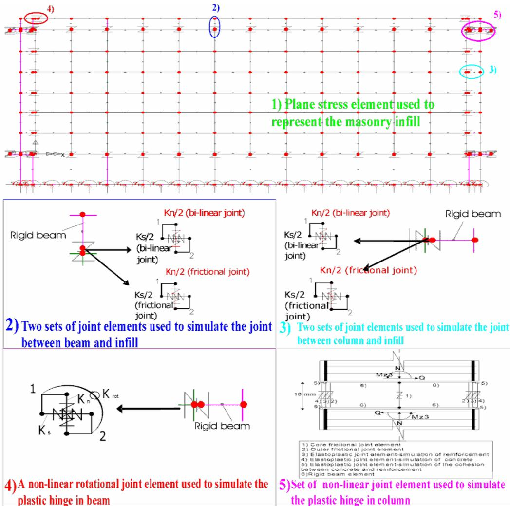
Figure 1. Fully non-linear numerical simulation of masonry infilled R/C model
