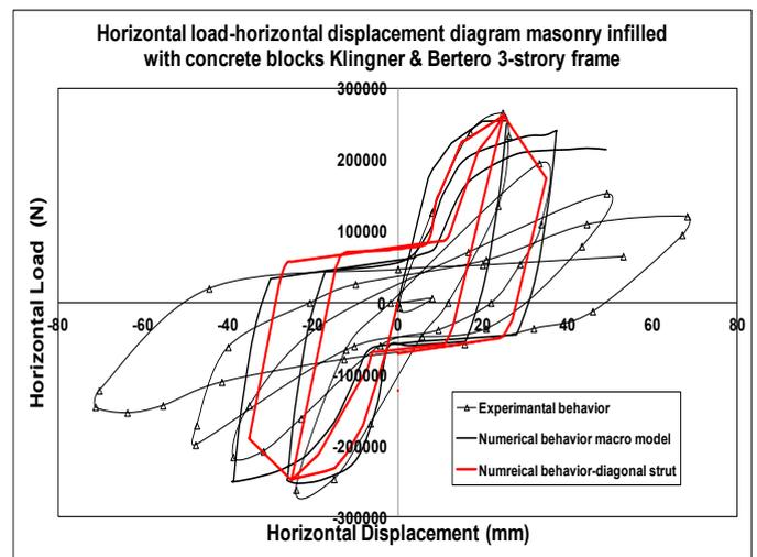
Figure 19. Comparison of cyclic response for Klingner & Bertero[10] 3-story masonry infilled frame with concrete blocks
