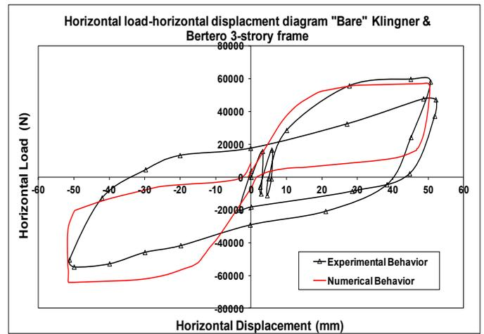
Figure 18. Comparison of cyclic response for Klingner & Bertero[10] 3-story “bare” frame
