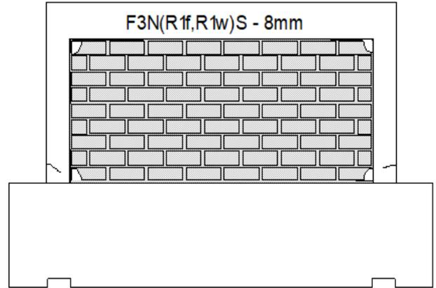
Figure 8. Experimental failure of masonry infilled frame F3N(R1f,R1w)s (Corner crushing)
