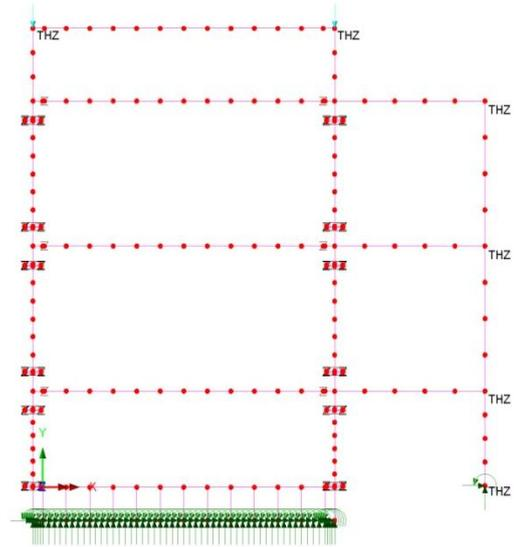
Figure 14. Numerical Simulation of the “bare” three story R/C frame
