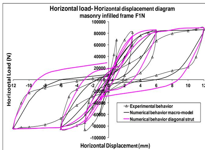
Figure 3. Comparison of cyclic response for specimen F1N
