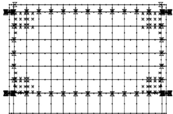
Figure 9. Failure predicted through macro-modeling technique
