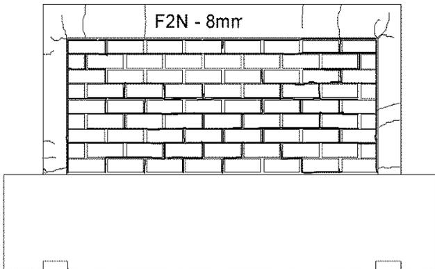
Figure 6. Experimental failure of masonry infilled frame F2N (DIAGONAL CRACKING)
