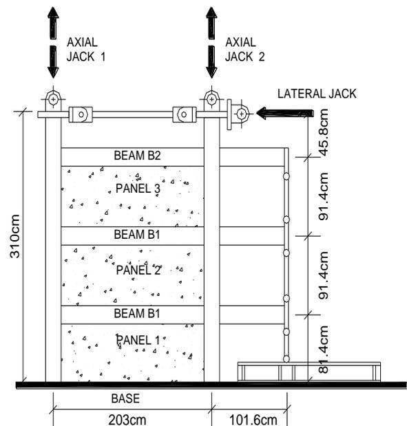
Figure 11. Masonry infilled R/C frame specimen [10]
