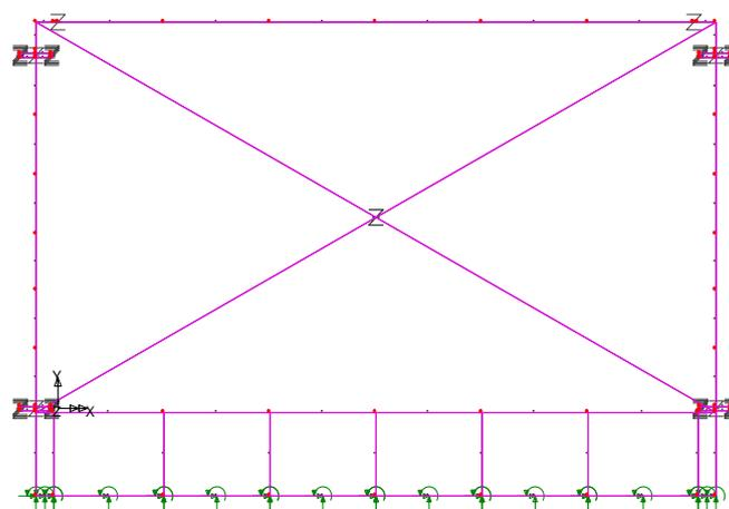
Figure 2. Equivalent diagonal strut model
