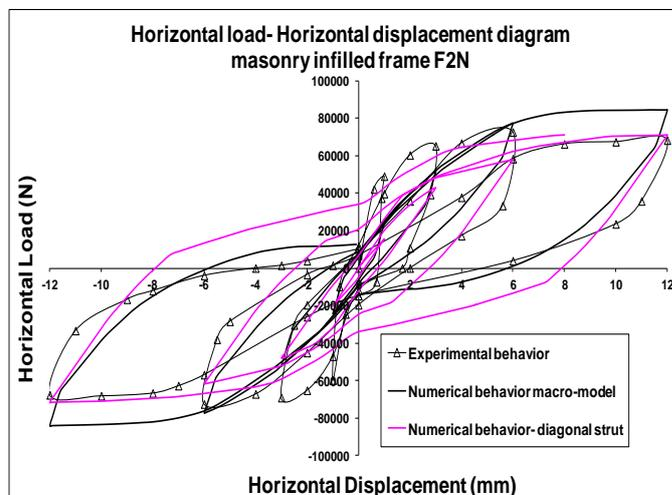
Figure 4. Comparison of cyclic response for specimen F2N
