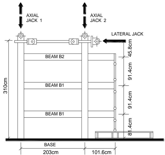
Figure 10. Bare frame specimen[10].
