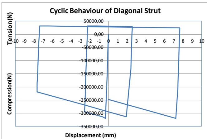
Figure 17. Hysteretic behaviour for the Klingner nad Bertero [10] equivalent diagonal strut
