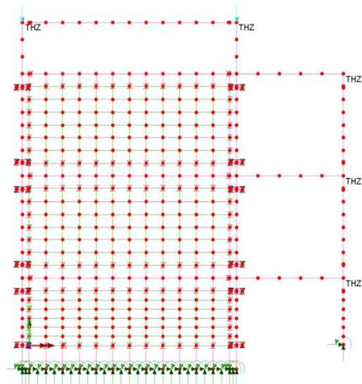
Figure 15. Numerical simulation of the three story masonry infilled R/C frame
